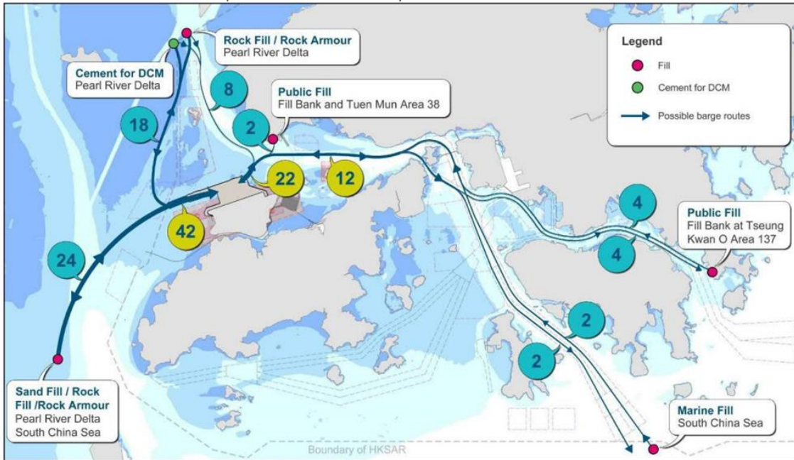
Figure 5-3: Indicative Marine Travel Route with Forecast Construction Traffic Movements on Average per Day After Commencement of Reclamation Before I-2RS (modified from BMT, 2014)
